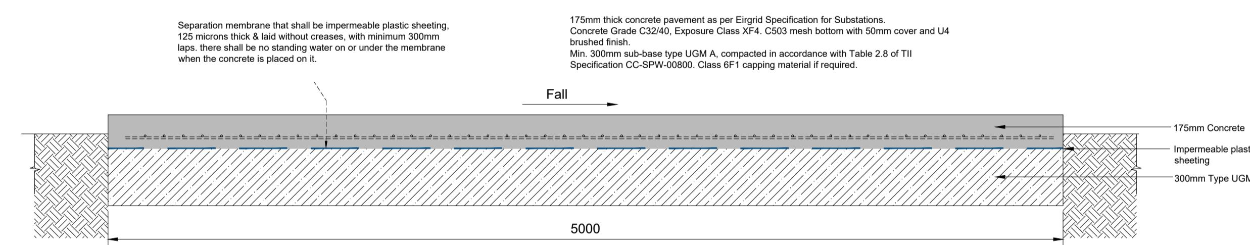
Substation Internal Road - Typical Detail
